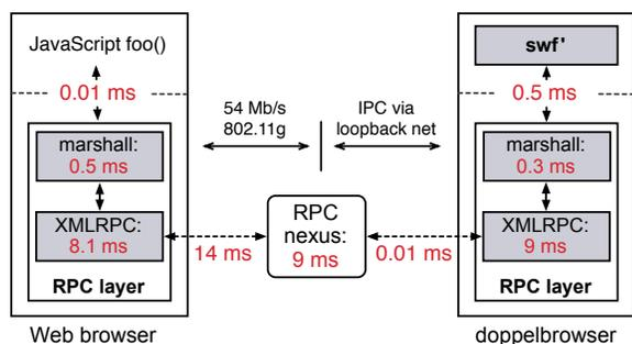
**Figure 7: Flash-to-JavaScript RPC overhead.** The total call time from (including return) from Flash to a remote JavaScript function is 41.4 ms, compared to 0.46 ms for a direct call from Flash to JavaScript on the same browser.
