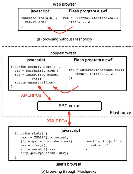
**Figure 3: JavaScript invocation.** (a) A Flash program can use `ExternalInterface` to call JavaScript functions. (b) FlashProxy rewrites Flash programs to call instead a stub JavaScript function on the doppelganger web page. This stub marshals the request and relays it through an “RPC nexus” process to a corresponding skeleton function that FlashProxy inserted on the user’s Web page. The skeleton invokes the appropriate JavaScript function.
