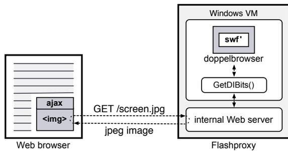
**Figure 5: Remote display.** Flashproxy uses the `GetDIBits` Windows system call to grab screenshots of the Flash program executing in the doppelbrowser on a Windows VM. The remote display AJAX component on the user's browser pulls screenshot updates from the Flashproxy internal Web server.
