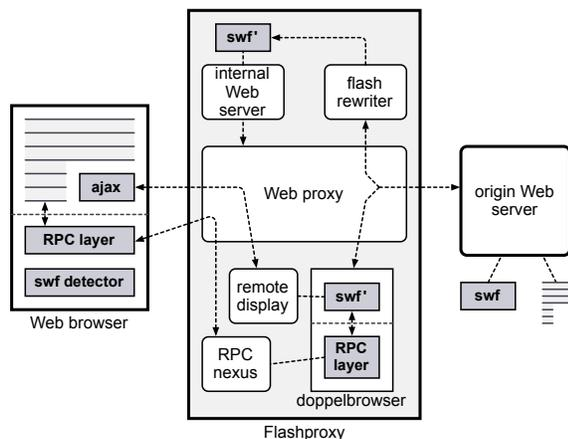
**Figure 4: Detailed Flashproxy architecture.** This diagram illustrates the additional components we needed to add to Flashproxy to handle a Flash program’s external interactions in a way that is transparent to both the user’s browser and the origin Web server.
