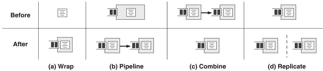
Fig. 3. *The four design patterns.* The four design patterns, *wrap*, *pipeline*, *combine*, and *replicate*, can be applied to stages of a service to condition it against load, failures, and limited or bottleneck resources.
