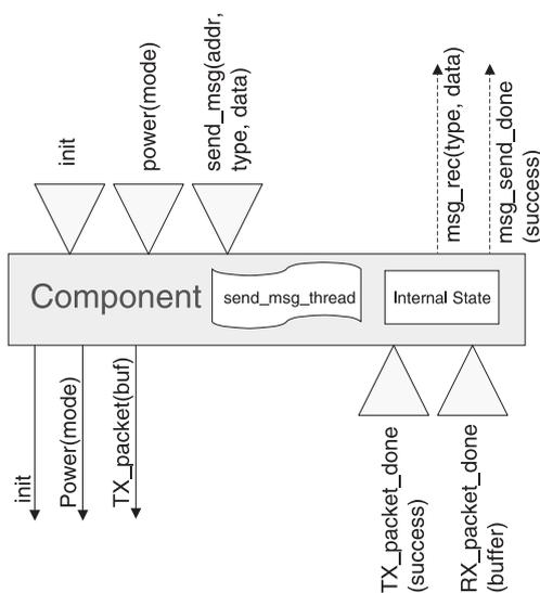
Fig. 9. A TinyOS software component. Each TinyOS software component accepts and emits commands and events. Commands flow from higher level layers to lower levels, and events flow from lower level layers to higher levels.
