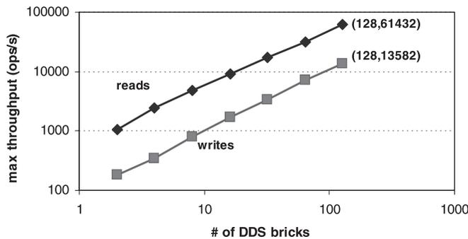
Fig. 6. Throughput scalability. This benchmark shows the linear scaling of throughput as a function of the number of bricks serving in a distributed hash table; note that both axis have logarithmic scales. As we added more bricks to the DDS, we increased the number of workers using the DDS until throughput saturated.
