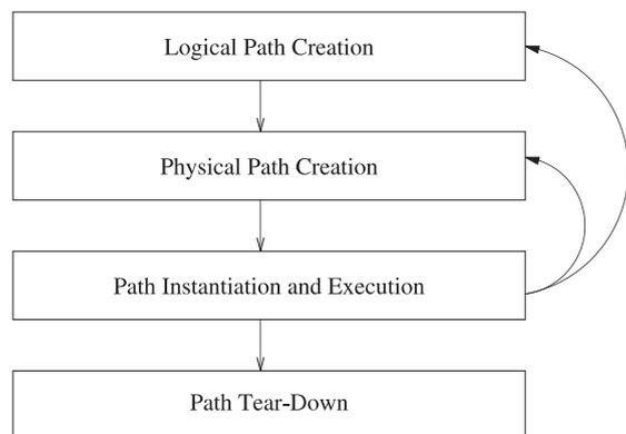
Fig. 11. *Path construction process.* Path execution is an iterative process of optimization. The Ninja APC facility guarantees the availability and fault-tolerance of a constructed path by rebuilding its physical or logical path.
