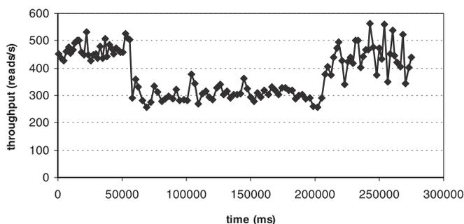
Fig. 7. *Availability and recovery*. This benchmark shows the read throughput of a three-node hash table as a deliberate single-node fault is induced, and afterwards as recovery is performed.
