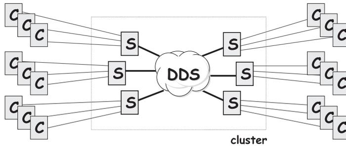
Fig. 5. High-level view of a DDS. A DDS is a self-managing data repository running on a cluster of workstations. All service instances (S) in the cluster see the same consistent image of the DDS; as a result, any WAN client (C) can communicate with any service instance.
