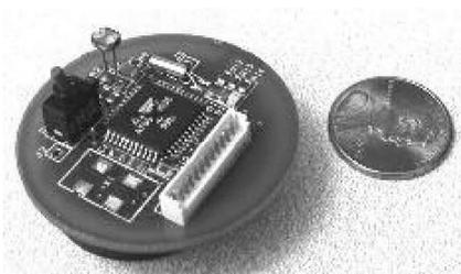
Fig. 8. A TinyOS-based mote. This “mote” includes a 4 MHz microcontroller, a software-driven radio, and an application that coordinates with neighboring motes to discover an ad hoc sensor network routing topology.
