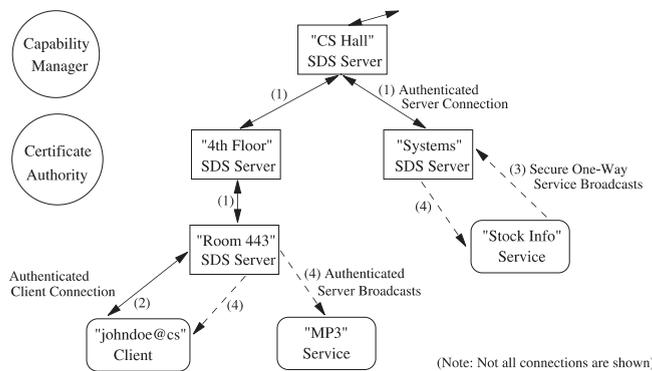
Fig. 10. Components of the Berkeley SDS. Dashed lines correspond to periodic multicast communication between components, while solid lines correspond to one-time transport connections.
