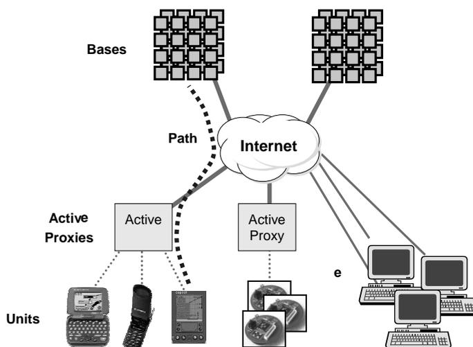
Fig. 1. *The Ninja platform architecture.* The architecture consists of bases (services running on clusters of workstations), active proxies (stateless or soft-state intermediaries between units and services), units (heterogeneous devices and sensors), and paths (a composition chain across units, proxies, and services in bases).
